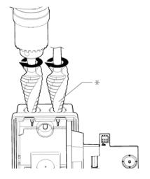
\*For the installation of the pressure relief plug for outdoor mounting
