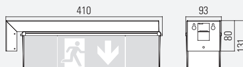
L01A WALL BRACKET MOUNTING
